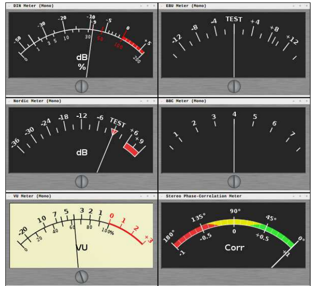
Figure 2. Various meter-types from the meter.lv2 plugin bundle fed with a -18 dBFS 1 kHz sine wave. Note, bottom right depicts the stereo phase correlation meter of a mono signal.
