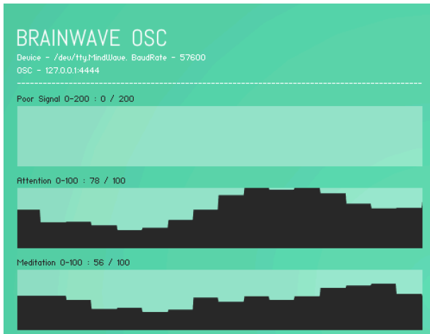
Figure 1. Screenshot of the BrainWave interface window, displaying the attention and meditation signals over a period of time. This data, along with the rest of EEG signals, is sent by this program over the network using the OSC protocol.
