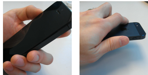
Figure 4. Gravity Y gesture (on the left), which is used for controlling note velocity, leading to a smaller velocity with a larger angle to the horizontal plane; Gravity Z gesture (on the right), which is used for quitting the current keyboard to reset everything again
