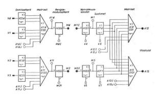
**Figure 2**: Block diagram of the DIMI-6000 signal path [5]
